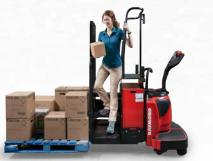
3 steps are designed with heavy-duty non-slip grating for enhanced stability in wet environments.
