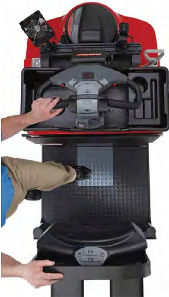
Roomy compartments include a curved back pad, knee pad, convenient lean points and operator-friendly rear controls, to ensure operator comfort throughout the shift.
