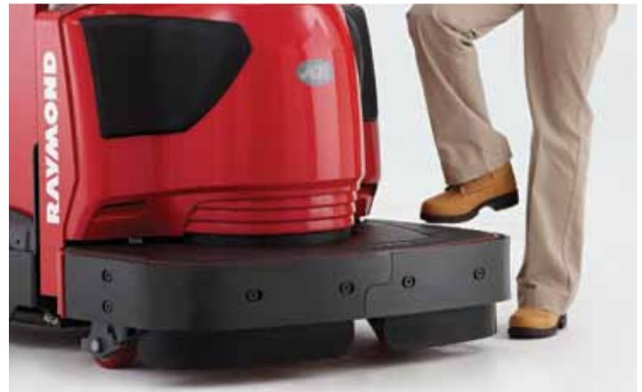
The roomy platform and low step height reduce operator fatigue.
