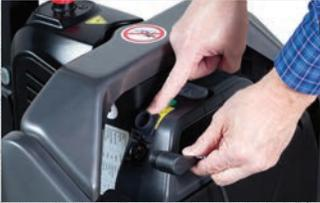
Charging port location allows battery to be charged inside or outside of truck
